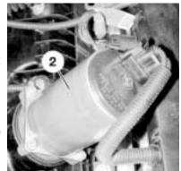
Valvetronic Sensors: Each eccentric shaft is monitored by a magneto-resistive position sensor. The N62 engine has two sensor assemblies, one for each eccentric shaft. These sensors are very durable for the environment (inside the cylinder head) and cope well with vibrations and high temperatures. The sensor assembly consists of:
